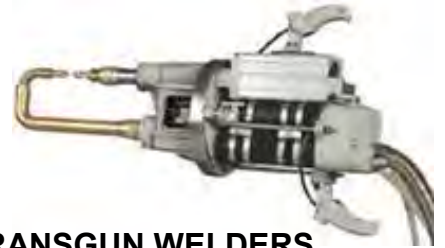
TYPICAL TRANSGUN WELDERS WELDING TRANSFORMER IS BUILT INTO THE WELDING GUN.
